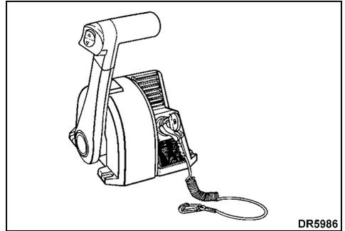
**IMPORTANT:** When shifting from FORWARD to REVERSE or from REVERSE to FORWARD, pause at NEUTRAL until the engine is at idle speed and the boat has slowed.
