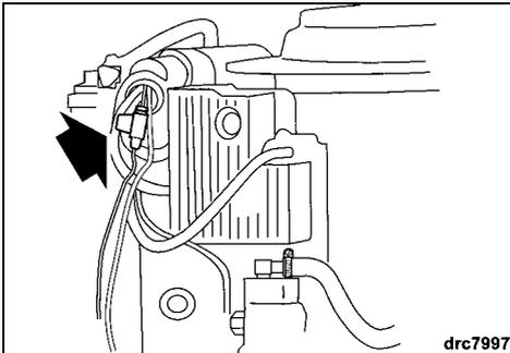
**IMPORTANT:** Failure to install cover securely will cause electrical problems.
