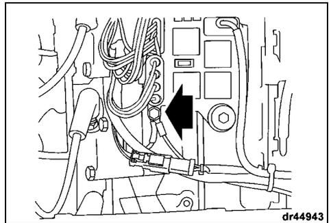
**IMPORTANT:** The accessory battery connection must only be used to charge a single 12-volt battery or two 12-volt batteries wired in parallel. The accessory connection must not be used to charge either battery in a 24-volt system.
