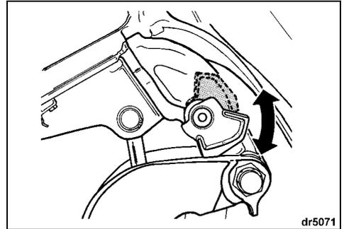
**Disengage** the tilt support lever:
