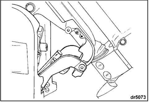
**To disengage bracket** — Tilt the motor fully. Return the trawling bracket to its stowed position. Lower the motor to its vertical position.
