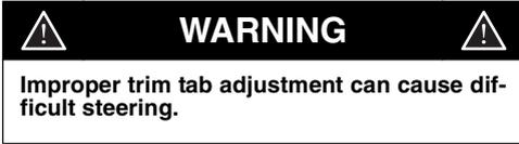
A propeller will generate steering torque when the propeller shaft is not running parallel to the water's surface. The trim tab is adjustable to compensate for this steering torque.
