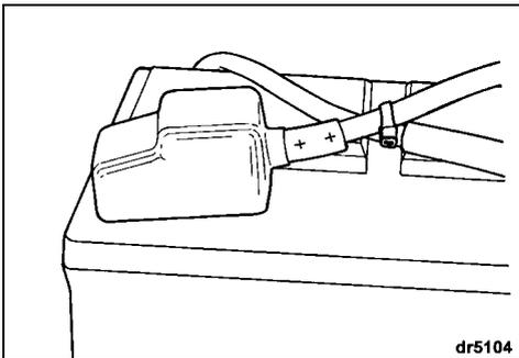
**IMPORTANT: DO NOT** use wing nuts on battery connections even if they came with the battery. Wing nuts can loosen and cause errant warning signals or electrical system damage.
