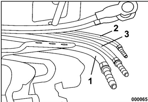
1. Fuel hose and fuel fitting - 3/8 in. (9 mm)
