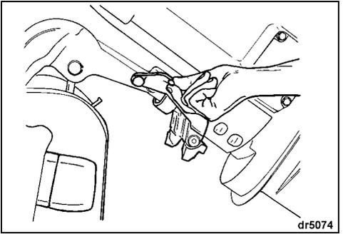
Pull down the trawling bracket. A detent will hold the bracket in position. Lower the motor until the trawling bracket locks into place in the stern brackets.
