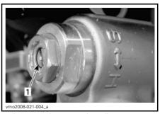
Low speed compression adjuster (flat screwdriver)
