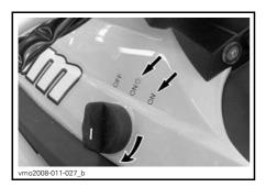
Place the emergency engine stop switch to RUN position.
