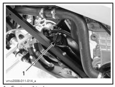
1. Engine oil tank cap
