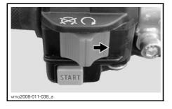
Shift transmission to NEUTRAL position or press and hold clutch lever.
