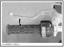
Press and hold engine start button until engine starts.
