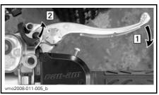
Step 1: Squeeze front brake lever and maintain Step 2: Move parking brake lever to desired position
