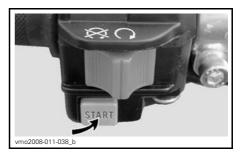
Release button immediately when engine has started.
