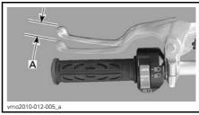
CLUTCH LEVER — PROPER ADJUSTMENT A. 10 mm to 15 mm (.39 in to .59 in)
