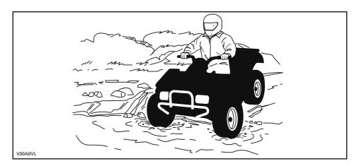
Water will affect the braking ability of your vehicle. Make sure you dry the brakes by applying them several times after the vehicle leaves the water.
