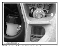
TYPICAL - DS 450/DS 450 X XC 1. Low speed compression adjuster (flat screwdriver)
