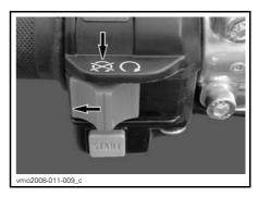
Turn ignition key to OFF position and remove key.
