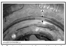
A. Gap (must be equal all around the wheel)
