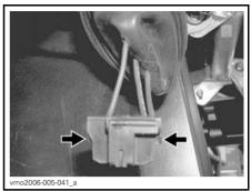
PUSH ON LOCKING TAB TO UNLOCK CONNECTOR
