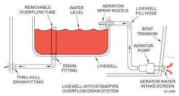
To use the aerated livewell, first install the drain plug or standpipe. Activate the switch labeled AERATOR on the dash or bow panel to pump water through the spray head and fill livewell. Turn off the pump when the livewell is sufficiently full. Note that the livewell will not fill unless you are stopped or going slowly. This is normal operation.
