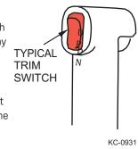
While monitoring the trim gauge, activate the trim and tilt function by pushing and holding the trim switch until the motor is at the desired angle.
