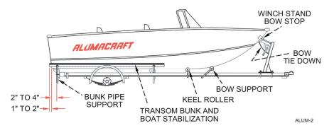
Position the carpeted bunks as far apart as practical. Pull the boat onto the trailer until the bunk pipe is within approximately 2 to 4 in. [5.1 to 10.2 cm] of the transom, and the bunks extend 1 to 2 in. [2.5 to 5.1 cm] beyond the transom. If the boat is loaded further back than this, the excess weight could cause the bunk supports to slip violently, causing damage to the hull. This will void the warranty.
