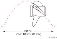
Pitch is the angle of the blades expressed in the theoretical distance a propeller travels in each revolution. In the above example, the pitch is 19, or each revolution of the propeller pushes the boat 19 in. [48.3 cm] through the water.
