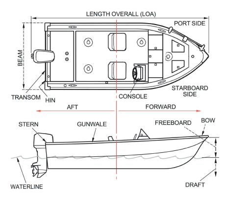
An easy way to distinguish port from starboard is to remember that "port" and "left" both have four letters.
