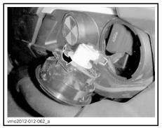
ROTATE BULB COUNTERCLOCKWISE
