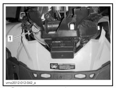
1. Engine coolant reservoir cap
