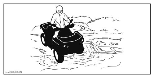
Water will affect the braking ability of your vehicle. Make sure you dry the brakes by applying them several times after the vehicle leaves the water. Allow greater distance for braking.
