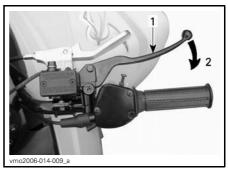
1. Brake lever 2. To apply brake
