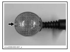
Tilt lens as shown to unlock it from housing.
