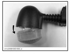
Push bulb in while turning it counterclockwise to release bulb from its socket.
