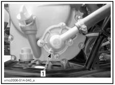
1. Cooling system drain plug
