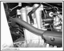
I H SIDE OF ENGINE 1. Air injection valve
