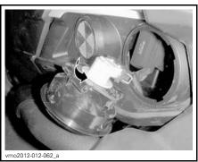
ROTATE BULB COUNTERCLOCKWISE
