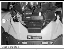
1. Engine coolant reservoir cap
