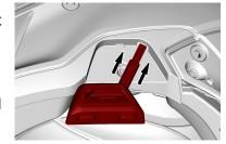
**6.** Make sure the user interface tab next to the wire is locked into the rectangular hole.
