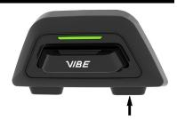
Hold the configuration button for 3 sec to access the configuration menu. You can then go to vehicle pairing by tapping the "up" button twice. Tap the center button to select "vehicle pairing". Then, on your vehicle display, go to Bluetooth settings and select your vibe product in the list of available devices.
