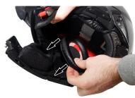
**A.8.** Reconnect the speaker cable with the BLACK female connector from the main unit. Repeat on the other side.
