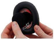
**A.7.** Reinstall the NCS into the helmet, making sure the openings are at the base of the helmet and the speaker cable is pointing toward the back of the helmet.
