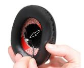
**A.6.** Using the Velcro, position and fix the speaker inside the NCS.
