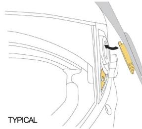
2. Once the tab is in position, pull the lever of the face shield mechanism downwards and slightly push the lower portion of the face shield to set the lower tab back in position.
