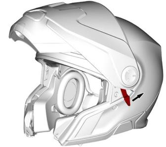
2. Insert the sun visor between helmet inner and outer shell and fit it on to the locating pegs on both sides.
