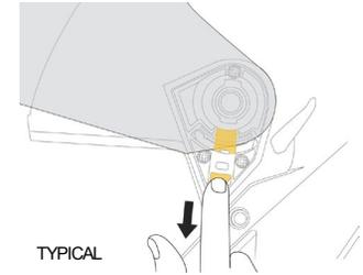
6. Move the lower portion of the face shield pivots upwards until the lower tab is released from the face shield mechanism.
