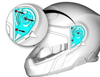
2. Use a Phillips #1 screwdriver to remove the three screws.
