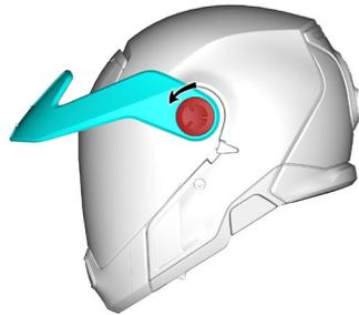
2. If helmet is equipped with a peak. Pull perpendicularly on the side of the peak as shown.
