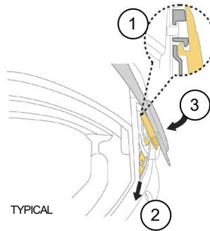
3. Then, release the lever. Make sure the spring pushes it back to the up position and check if the visor is correctly held in place.
