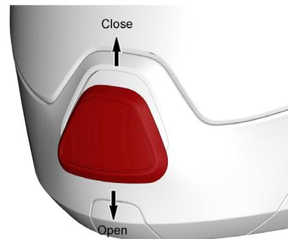
2. **OPEN:** The lower vents are adjustable in 3 positions. When placing both sliding buttons on the «
