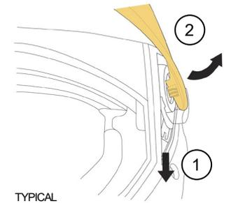
7. Then, pull the face shield downward to release the upper tab from the face shield mechanism.
