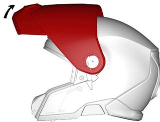
5. On one side, pull the lever of the face shield mechanism downward to release the lower tab of the face shield.
