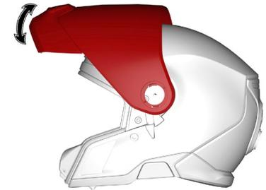
6. Make sure that the face shield mechanism is functioning properly by closing and opening the face shield to its maximum extent.
