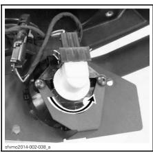
TYPICAL: ROTATE BULB COUNTERCLOCKWISE
