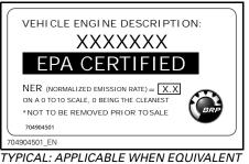
TYPICAL: APPLICABLE WHEN EQUIVALENT TO A MODEL CERTIFIED TO US EPA STANDARDS
