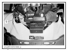
1. Engine coolant reservoir cap
