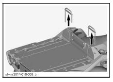
3. Place side wall on flat bed and lower it on its place.
