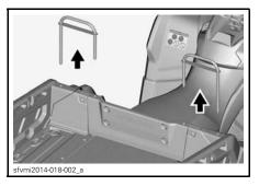
5. Lift side wall up and remove it. Repeat on other side.
