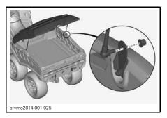
3. Remove pins from hinges both sides.
