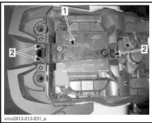
Battery holder 2. Retaining screws
