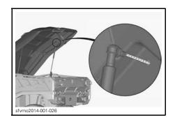
2. Detach the lower end by removing nut.
