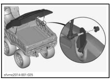
9. Install the shock's top end by screwing it into place.
