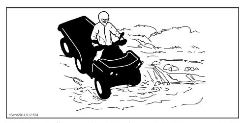
Wet brakes will affect the braking ability of your vehicle. Make sure you dry the brakes by applying them several times after the vehicle leaves the water, mud or snow. Allow greater distance for braking.
