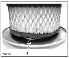
1. Gap between filter and filter base
