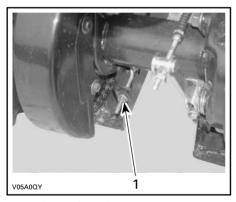
**4-STROKE MODELS**1. Drive chain adjusting nut
