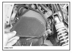
To clean the air filter element use the following procedure.
