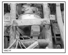
bolts (one on each side of air filter box cover)
