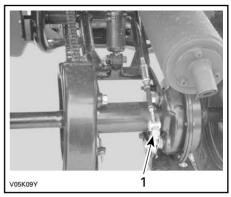
**4-STROKE MODELS**1. Adjusting nut
