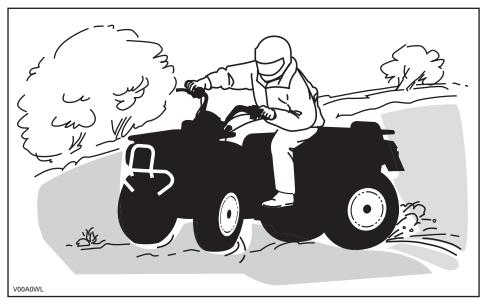
If you do get into a slide or skid, it may help to turn the handlebar into the direction of the skid until you regain control. Never jam the brakes and lock the wheels. Respect and follow all posted trail signs. They are there to help you and others.
