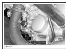
Remove oil filter and replace with a new filter.
