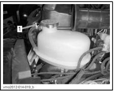
1. Engine coolant reservoir cap
