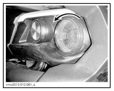
Disconnect the light bulb connector. Rotate light bulb counterclockwise to remove it from taillight.
