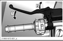
Step 1: Apply brakes Step 2: Lock brakes
