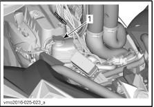
1. Engine coolant reservoir cap
