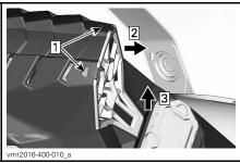
Step 1: Push down on tabs Step 2: Gently pull top of grille out Step 3: Pull bottom of grille up
