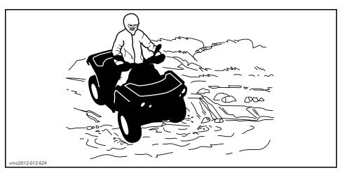
Water will affect the braking ability of your vehicle. Make sure you dry the brakes by applying them several times after the vehicle leaves the water.
