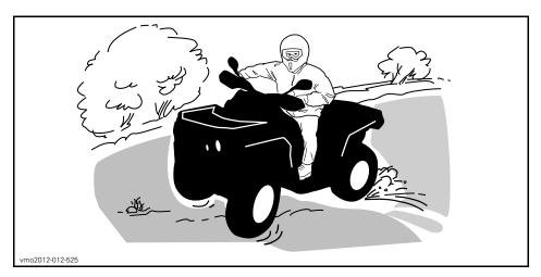
If you do get into a slide or skid, it may help to turn the handlebar in the direction of the skid until you regain control. Never jam the brakes and lock the wheels.
