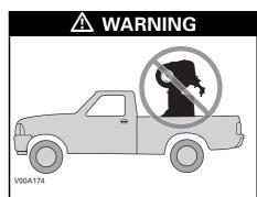
Never tip this vehicle on end for transporting. We recommend that you carry the vehicle in its normal operating position (on all four wheels).
