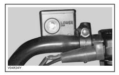
Visually inspect lever boot condition. Check for cracks, tears etc. Replace if damaged.
