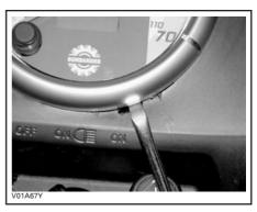
Plug connectors to change units from miles to kilometers. Unplug to return to miles reading.
