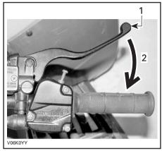
1. Brake lever 2. To apply brake
