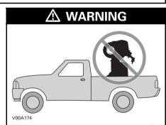
Never tip this vehicle on end for transporting. We recommend that you carry the vehicle in its normal operating position (on all 4 wheels).
