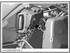
TYPICAL — RH SIDE OF ENGINE COMPARTMENT 1. 5 A main fuse
