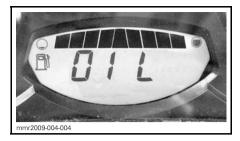
The engine lubrication procedure takes approximately 1 minute. During this time the engine RPM will increase slightly.
