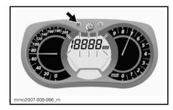
Push and hold the SET (S) button within 5 seconds to reset.
