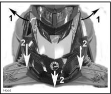
Step 1: Step 1: Release retaining pins Step 2: Step 2: Slide hood towards the front
