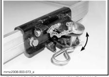
HITCH MOVES FREELY WHEN TOWING
