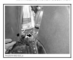
To remove a side panel, open it then lift it up. Free the lower hinge from its slot, then free the upper hinge by lowering the panel.
