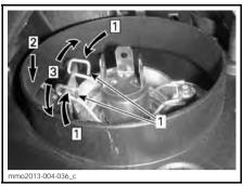
Step 1: Push both sides Step 2: Push down to release Step 3: Release both sides
