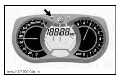
While display is flashing, press the SET (S) button to select speedometer mode.
