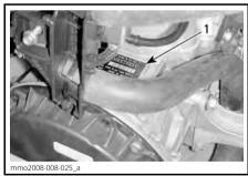
600 HO E-TEC® ENGINE — RH SIDE OF ENGINE COMPARTMENT 1. Engine serial number
