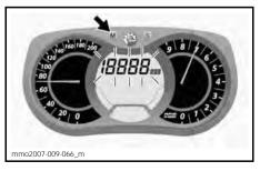
While display is flashing, press SET (S) button to select RPM mode.
