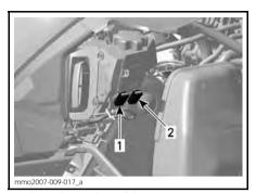
RH SIDE OF ENGINE COMPARTMENT 15 A headlight fuse (RED/ORANGE wire) 15 A accessories fuse (RED/YELLOW wire)
