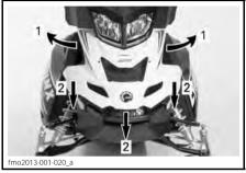
Step 1: Step 1: Release retaining pins Step 2: Step 2: Slide hood towards the front
