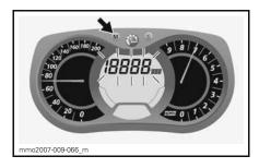
While display is flashing, press SET (S) button to select RPM mode.
