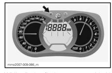
While display flashes, press and hold the SET (S) button within 5 seconds to reset
