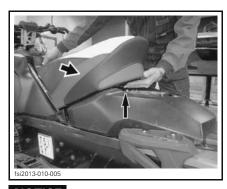
**NOTICE** Pull the handle upwards when removing the seat.
