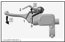
TYPICAL — ENGAGE MECHANISM Step 1: Step 1: Squeeze and maintain brake lever Step 2: Step 2: Adjust locking lever
