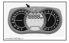
While display flashes, press SET (S) button to select vehicle average speed (AVR\_SPD) mode.
