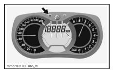
While display flashes, press the SET (S) button to select top speed (TOP\_SPD) mode.
