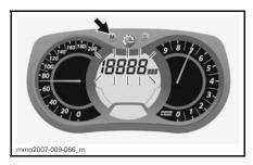
While display flashes, press the SET (S) button to select total fuel consumption (TC) mode.
