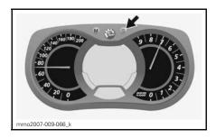
To change HOURS, while the value of HOURS is blinking, use the SET (S) button to change hours.
