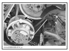
Pull the rope using a sharp, crisp pull so the rope comes free of the drive pulley. Start engine as per usual manual starting.
