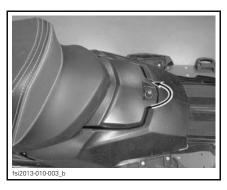
Remove the seat by pulling and lifting at the same time.
