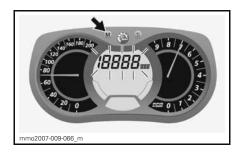
While display is flashing, press the SET (S) button to select altitude mode.
