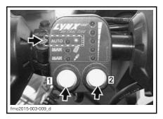
To use preselected values push the left button till AUTO led lights up. Push the right knob to set the preselected spring preload and damping force. Upwards is more spring preload/damping force and down is less spring preload/damping force.
