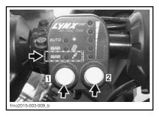
To increase or decrease the damping push the left knob till the MAN/shock figure led lights up. Push the right knob to set the damping. Upwards is more damping and down is less damping.
