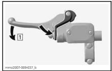
TYPICAL — RELEASE MECHANISM Step 1: Step 1: Squeeze brake lever
