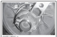
ALUMINUM ADJUSTER HUB 1. Suspension adjustment tool
