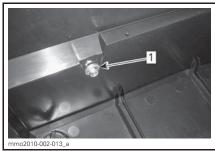
*INSIDE THE STORAGE BOX* 1. Retaining screw
