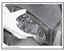
3. Unplug burnt bulb connector. Remove the rubber boot.
