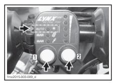
To use preselected values push the left button till AUTO led lights up. Push the right knob to set the preselected spring preload and damping force. Upwards is more spring preload/damping force and down is less spring preload/dampina force.
