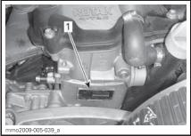
1200 4-TEC ENGINE 1. Engine serial number
