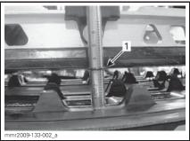
1. Deflection O-ring aligned with slider shoe
