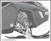
TYPICAL - CAM TYPE PRELOAD 1. Adjustment cam
