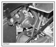
Insert the needle of lubricant can in the end of throttle cable adjuster.
