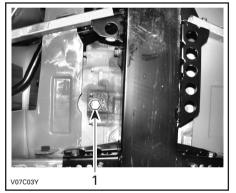
TYPICAL 1. Oil drain plug Allow enough time for oil to flow out of oil filter. Remove the right engine cover. Unscrew the oil filter cover.
