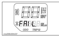
If your speedometer shows FAIL in the multifunction display, it means that the speedometer as sensed 18 volts in the electrical system, caused by a disconnected or defective voltage regulator.
