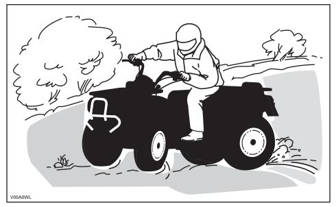
If you do get into a slide or skid, it may help to turn the handlebar into the direction of the skid until you regain control. Never jam the brakes and lock the wheels.
