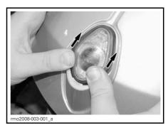
Lift front portion of lens with your thumb or a small screwdriver to release.
