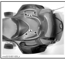
A. Different gripping positions on the handholds
