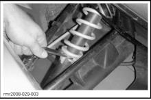
FRONT SUSPENSION CAM ADJUSTMENT
