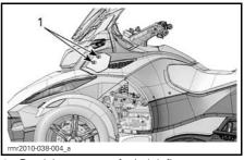
1. Retaining screws of wind deflector
