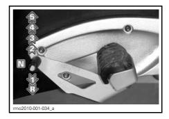
Lift up or press down fully to move sequentially from one gear to the next. When the lever is released, it returns to center where the mechanism resets for the next shift up or down. Neutral (N) is selected by either a half lift from first gear or a half press from second gear. Refer to 8) SHIFTING (p. 67) for detailed instructions.
