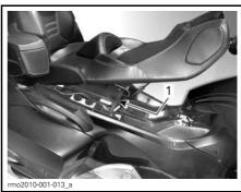
1. Fuse box located under the seat
