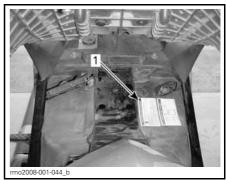
EPA exhaust emission label located under seat
