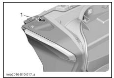
1. Upper retaining screw to remove
