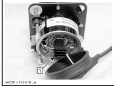
Step 1: Remove connector from light bulb
