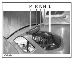
To change the transmission position, completely stop vehicle then move lever to the right then to the desired position while moving lever forward. Do not force lever. If unable to shift, gently apply throttle to move ATV and try again.
