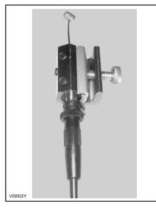
Insert the needle of lubricant can on the cable luber hole.
