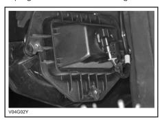
Rotate the bulb socket counterclockwise then remove headlight.
