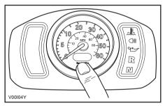
Press once to switch from odometer to tripmeter or vice versa. Press and hold to reset while in trip meter selection.
