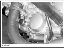
Remove the oil filter and replace by a new filter.
