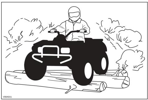
Even though there is an adequate suspensions system on an this vehicle there are "washboard" or rough terrain conditions that will make you feel uncomfortable and even cause back injury. "Posting" or riding in a crouched position will often be required. Slow down and allow your flexed legs to absorb impact.
