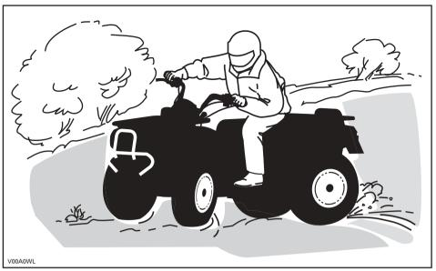
If you do get into a slide or skid, it may help to turn the handlebar into the direction of the skid until you regain control. Never jam the brakes and lock the wheels.
