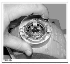
Lift and hold the spindle then remove the bulb.
