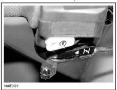
Press start button and hold until engine starts. **CAUTION:** Do not hold start button more than 30 seconds. A rest period should be observed between the cranking cycles to let starter cool down. Pay attention not to discharge battery.
