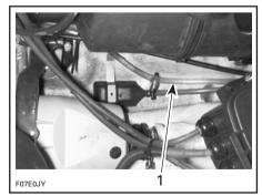
1. Engine cylinder drain hose
