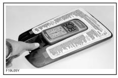
To reinstall, position GPS receiver in its receptacle and push until it latches.
