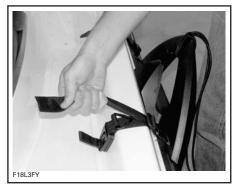
Double-check that rack is properly installed by giving it a tug.
