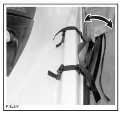
**NOTE:** When wakeboard is removed from its rack, secure bungee cords so that they will not move freely when riding watercraft.
