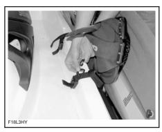
After installation, pull and push wakeboard to ensure it is tightly secured to rack.
