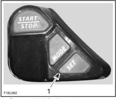
1. Press and hold for 2 seconds to reset
