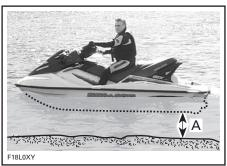
A. Maintain at least 90 cm (3 ft) underneath the lowest rear portion of the hull when all passengers are aboard
