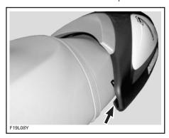
Finish pushing cover in position then lock the quarter-turn screws.
