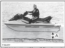
Maintain at least 90 cm (3 ft) underneath the lowest rear portion of the hull when all passengers are aboard
