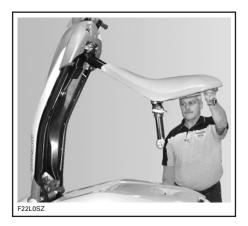
Rotate the post to a vertical position and move the seat to line up the post with its receiver.
