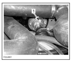
1. Grease seal carrier of mid bearing
