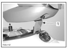
1. Steering pole retainer locked
