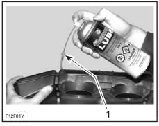
1. Partially pull tube out of air box to inject XP-S Lube lubricant or equivalent. Push tube in when finished.
