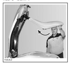
**CAUTION:** Make sure to maintain the steering pole high enough so that the "moto" seat clears the engine cover when rotated forward into the pole.
