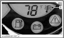
**TYPICAL — UNDER SPEEDOMETER** 1. Water temperature
