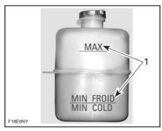
1. Level between marks when engine is cold
