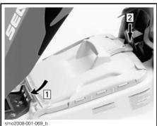
Step 1: Insert storage bin front tabs Step 2: Push to secure
