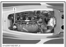
MODELS WITHOUT AN ENGINE COVER 1. Oil filling cap
