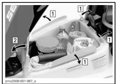
Step 1: Release cover latches Step 2: Open cover
