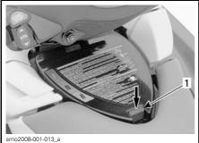
PUSH ON LATCH TO RELEASE 1. Cover latch
