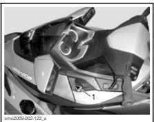
TYPICAL - STORAGE BIN ACCESS 1. Front cover latch handles (one each side)
