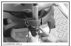
PUSH TOWARD FRONT TO UNLOCK AND REMOVE POST 1. Locking clip
