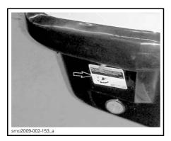
The 4-TEC<sup>TM</sup> engine features a tip-over protection system (T.O.P.S.<sup>TM</sup>). When the watercraft tips over, the engine is automatically stopped.
