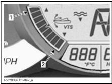
The VTS system allows for manually adjusting the trim position of the nozzle, or selecting two preset trim posi-tions and recording or changing preset trim positions on certain models.
