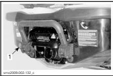
TYPICAL 1. Flushing connector
