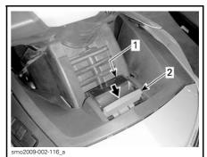
STEERING COLUMN ADJUSTMENT LATCH NOT SECURED
