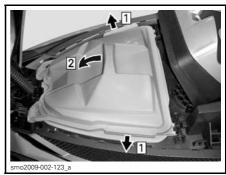
HOW TO OPEN STORAGE BIN Step 1: Release cover latches Step 2: Pull cover open
