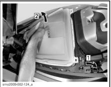
STORAGE BIN REMOVAL Step 1: Push back on storage bin latches Step 2: Lift and tilt forward to release front tabs
