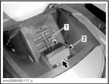
STEERING COLUMN ADJUSTMENT LATCH PROPERLY SECURED 1. Latch pawl engaged
