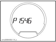
TYPICAL - ENGINE FAULT CODE DISPLAYED
