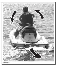
TYPICAL - STEERING DIRECTION REVERSED WHEN BACKING
