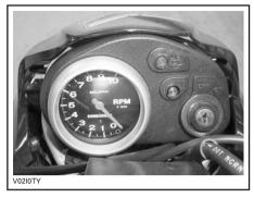
The tachometer indicates the revolution per minute (RPM) of the engine. Multiply by 1000 to obtain an approximation of the actual RPM.
