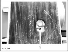
UNDER VEHICLE 1. Oil drain plug
