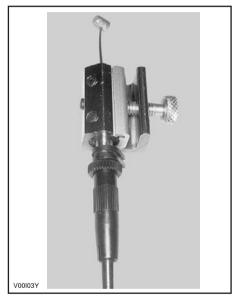
Insert the needle of lubricant can on the cable luber hole.
