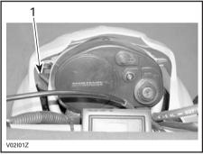
1. Engine/transmission oil tank cap
