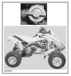
**CAUTION:** Improper opening of fuel valve will restrict the flow of fuel. Make sure valve is fully opened while running.
