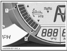
$\begin{array}{l} \textit{INFORMATION CENTER} - \textit{VTS POSITION} \\ \textit{INDICATOR} \end{array}$
