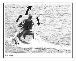
Turning the handlebar pivots the jet pump nozzle which controls the watercraft direction. Turning the handlebar to the right will turn the watercraft to the right and inversely. The throttle should be applied to turn the watercraft.
