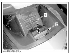
STEERING COLUMN ADJUSTMENT LATCH NOT SECURED
