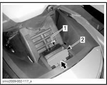
STEERING COLUMN ADJUSTMENT LATCH PROPERLY SECURED
