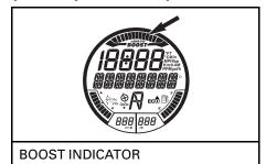
The boost gauge indicates the manifold pressure of the engine provided by the supercharger.
