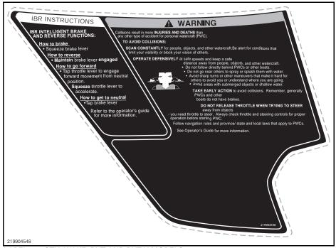
LABEL 16: GTX, WAKE, RXT AND RXT-X MODELS
