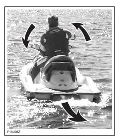
TYPICAL - STEERING DIRECTION REVERSED WHEN BACKING
