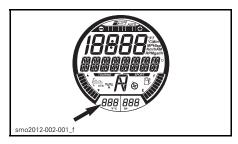
The numerical display may also be selected to display water temperature. See *NUMERICAL DISPLAY* in this section.
