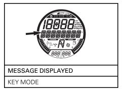
4. Press the SET button once to enable learning key mode setting function. The display will change to L-Key.
