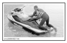
Take hold of the seat strap to help maintain your balance and step forward onto the footboards on either side of the seat.
