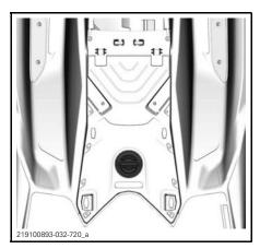
3. Remove engine service cover by removing the retaining screws.
