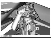
TYPICAL - PUSH TOWARD FRONT TO UNLOCK AND REMOVE PYLON
