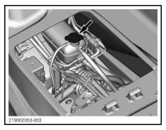
With watercraft on a level surface, coolant level should be between MIN. and MAX. marks on coolant reservoir when engine is cold.
