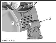
STEERING COLUMN ADJUSTMENT LATCH SECURED
