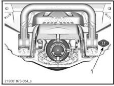
1. Flushing connector location
