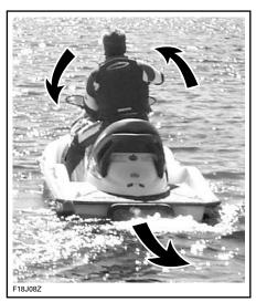
TYPICAL - STEERING DIRECTION REVERSED WHEN BACKING
