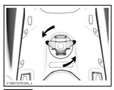
**NOTICE** It is very important to install the ski pylon hole cover to prevent water infiltration into the hull.
