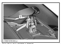
SKI PYLON RETRACTED 1. Pull on this knob to extend
