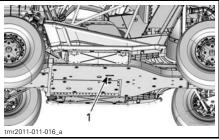
1. Cooling system drain plug access
