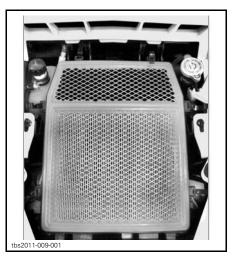
3. Verify that the cover fits well on the engine air filter housing before closing clamps.
