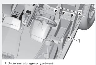
1. Under seat storage compartment 2. Plastic rivets
