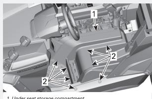
1. Under seat storage compartment 2. Plastic rivets
