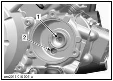
Outlet to the engine oil providing system
