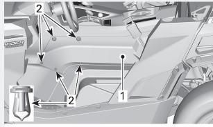
FRONT PORTION OF THE LH LATERAL CONSOLE PANEL LH lateral console panel
