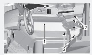
REAR PORTION OF THE LH LATERAL CONSOLE PANEL 1. LH lateraı co 2. Plastic rivets
