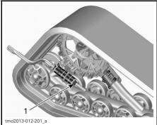
TYPICAL - REAR TRACK ASSEMBLY 1. Elastic nut
