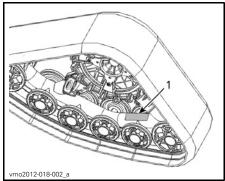
RH FRONT TRACK ASSEMBLY 1. Identification plate
