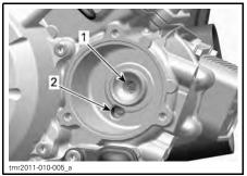
Outlet to the engine oil providing system
