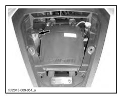
Coolant should be at the MIN mark when engine is COLD.
