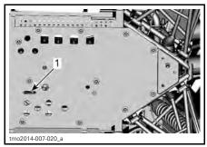
1. Cooling system drain plug access
