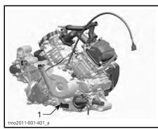
TYPICAL — ENGINE SERIAL NUMBER LABEL 1. EIN (Engine Identification Number)
