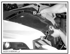
Step 1: Keep on lifting the front part of service cover Step 2: Gently release the cover post from its
