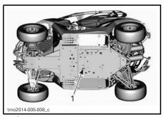
1. Cooling system drain plug access
