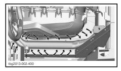
Using a garden hose, thoroughly clean the area so that no more debris can be in contact with the exhaust.
