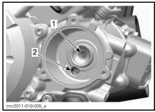
1. Outlet to the engine oil providing system
