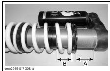
TYPICAL - CROSSOVER ADJUSTMENT -REAR SHOCK A. Spring preload B. Crossover ring position
