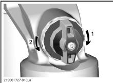
COMPRESSION DAMPING 1. Increases damping (stiffer)
