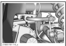
TYPICAL - FRONT STABILIZER BAR 1. Grease fitting
