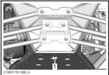
TYPICAL, REAR OF VEHICLE 1. Hydraulic jack position
