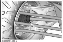
**REAR OF VEHICLE** 1. Outer drive shaft boot
