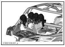
Remove air filter cap to let out any water that may have be introduced.
