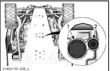
UNDERNEATH REAR OF VEHICLE 1. Magnetic drain plug 2. Secondary drain plug
