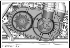
PARTS REMOVED FOR CLARITY 1. CVT cover
