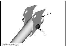
FRONT ADJUSTMENT MECHANISM IN POSITION LOW
