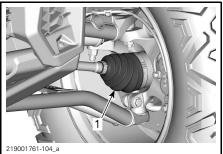
FRONT OF VEHICLE 1. Outer drive shaft boot
