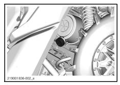
The snorkel grills can be removed for cleaning by removing the screw.
