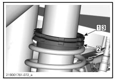
**TYPICAL** Step 1: Loosen top locking ring Step 2: Turn adjusting ring accordingly Step 3: Tighten top locking ring
