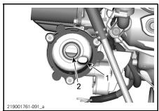
Outlet to the engine oil providing system
