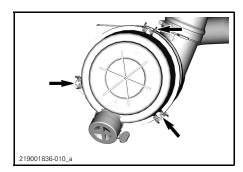
Remove the filter cartridge.
