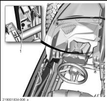
UNDERNEATH OF THE LH SIDE DASHBOARD 1 Plastic rivet
