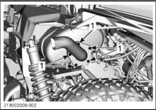
1. Tail pipe retaining screws
