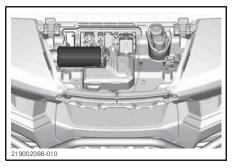
Lift and slide filter to remove.
