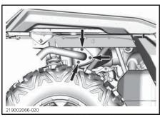
TAIL PIPE RETAINING SCREWS
