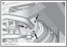
TAIL PIPE RETAINING BOLTS AND NUTS
