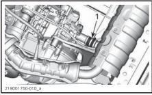
1. Propeller shaft bellows
