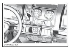
The differential switch enables locking of rear differential.
