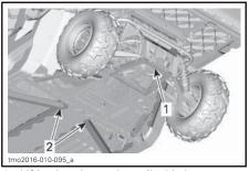
1. Lifting location under trailer hitch
