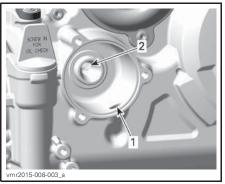
Inlet bore from the oil pump to the oil filter
