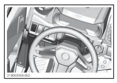
This switch is used to select either the headlights OFF position, low or high beams.
