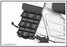
Clean air filter by washing it in lukewarm water with mild soap. Remove excess water and air dry before installation.
