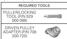
Insert adaptor in threaded hole of driven pulley then screw tool in the threaded hole of adaptor and tighten to open the pulley.
