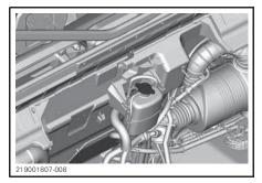
Unscrew coolant drain plug and drain the coolant into a suitable container.
