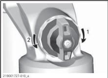
COMPRESSION DAMPING 1. Increases damping (stiffer)
