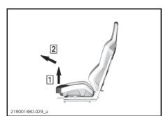
SEAT CUSHION Step 1: lift front of seat Step 2: Pull toward the front
