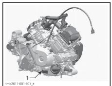
TYPICAL 800 AND 1000 — ENGINE SERIAL NUMBER LABEL 1. EIN (Engine Identification Number)
