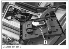
TYPICAL — FRONT ACCESS PANEL 1. Winch remote control
