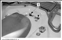
Holes for passenger's seat positioning tubes
