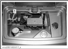
TYPICAL — FRONT SERVICE COMPARTMENT 1. Remote control connection
