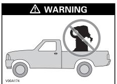
Never tip this vehicle on end for transporting. We recommend that you carry the vehicle in its normal operating position (on all four wheels).
