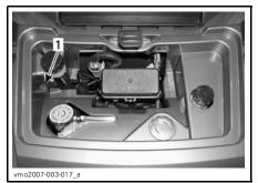
TYPICAL — FRONT SERVICE COMPARTMENT 1. Remote control connection
