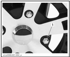
**TYPICAL — CLOSED END TYPE** 1. Wheel nut
