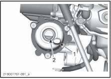
Outlet to the engine oil providing system
