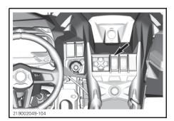
This switch selects 2 wheel drive or 4 wheel drive mode when the vehicle is stopped and the engine is running.
