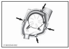
Remove the filter cartridge.
