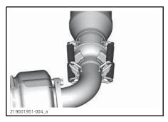
Pull out spark arrestor and remove carbon deposits using a brush.
