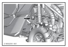
**NOTICE** If sand or other particles are found in air filter housing, clean it using a vacuum cleaner.
