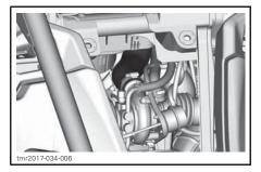
Open intercooler and crankcase hose support by removing the screw.
