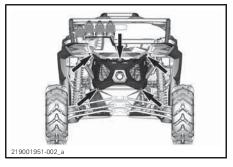
Remove and discard the retaining bolts and nuts.
