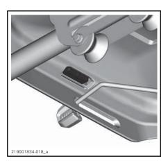
Pull up the rear of the cushion, then free the cushion from the seat frame by pulling it off towards the rear.
