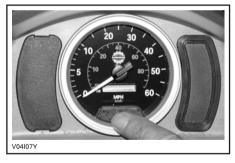
The odometer can indicate in miles or in kilometers. See an authorized Bombardier ATV dealer to change the indications.
