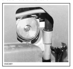
Remove the oil filter and replace with a new filter.
