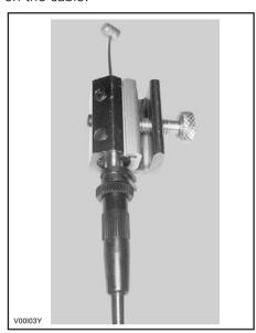
Insert the needle of lubricant can on the cable luber hole.
