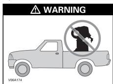
Never tip this vehicle on end for transporting. We recommend that you carry the vehicle in its normal operating position (on all four wheels).
