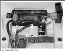
SERVICE COMPARTMENT UNDERNEATH SEAT 1. Tool kit
