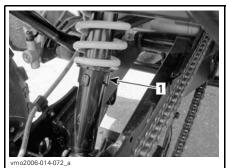
**REAR SUSPENSION** 1. Preload cam
