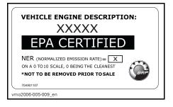
The following labels are on your vehicle and they should be considered permanent parts of the vehicle. If missing or damaged, they can be replaced free of charge. See an authorized Can-Am dealer.
