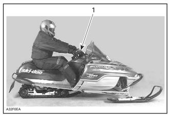
TYPICAL — GOOD ADJUSTMENT AT MODERATE SPEED 1. Handlebar easy to turn — neutral steering attitude
