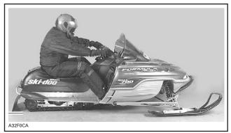
TYPICAL — TOO SOFT OF ADJUSTMENT (REAR SUSPENSION IS TOO LOW, IT HAS COLLAPSED MORE THAN 75 mm (3 in)
