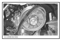
Remove drive belt from drive pulley.
