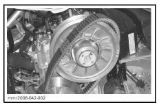
When drive belt is in position, driven pulley sheaves needs to be adjusted to obtain proper drive belt adjustment.
