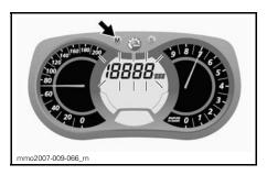
While display is flashing, press the SET (S) button to select altitude mode.
