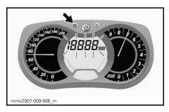
Press and hold the SET (S) button within 5 seconds to reset.
