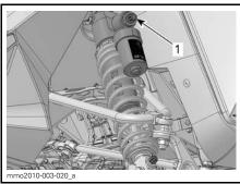
Low speed compression damping adjuster (slot or knob)
