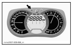
While display flashes, press SET (S) button to select vehicle average speed (AVR SPD) mode.
