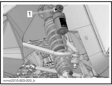
1. High speed compression damping adjuster (hexagonal)
