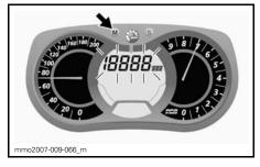
Press and hold the SET (S) button within 5 seconds to reset.
