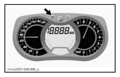
To reset maximum temperature recorded, press the MODE (M) to select mode.
